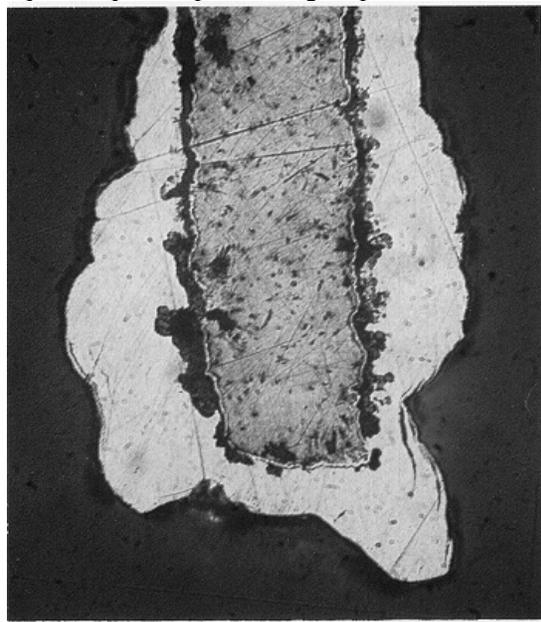
Figure 11. Rounded Nickel Deposits and Localized Loss of Adherence at an Overplated Edge (NiDU3, 180X)
