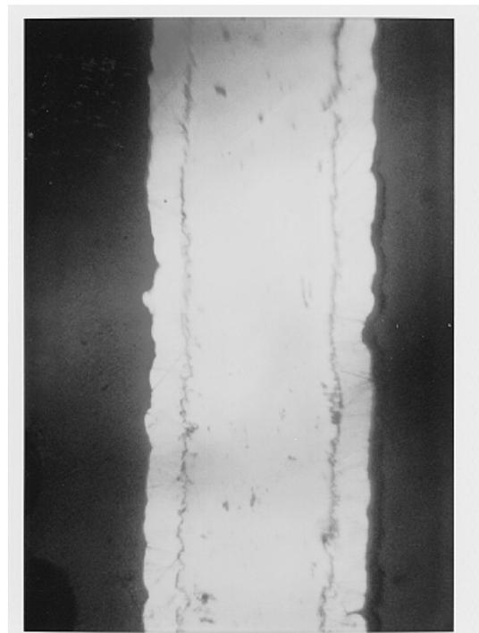
Figure 5. Uniform and Continuous Zinc Plating on a Properly Etched Adjusted-Uranium Substrate (ZnLEU24, 220X)
