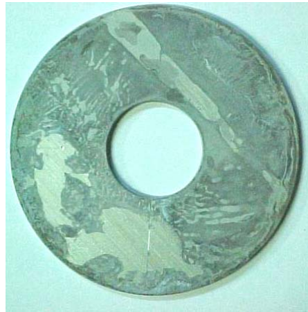
Fig. 9: Uneven oxidation (x 1)
