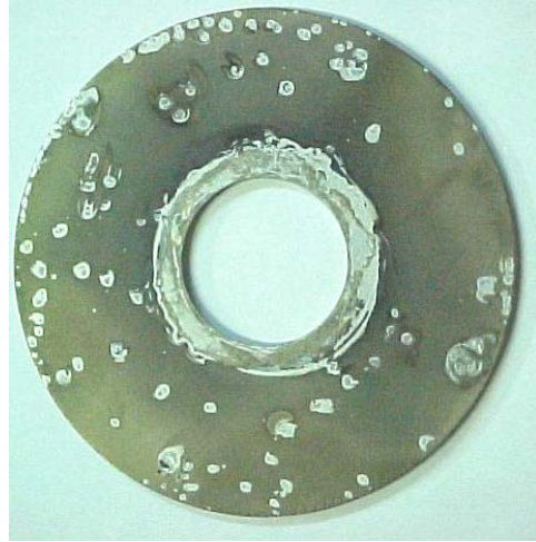
Fig. 10: Pitted surface (x 1)
