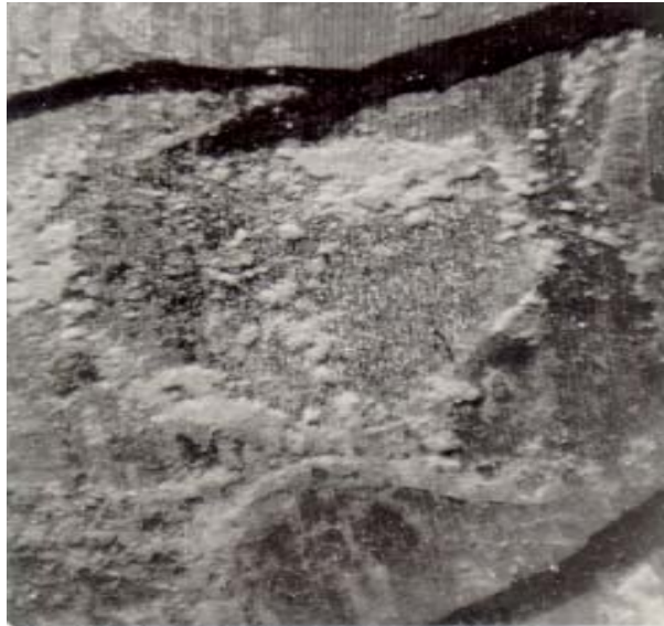
Fig. 7: Coupon 6064/64; crevice corrosion (18X)
