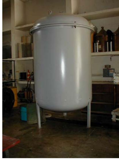
Figure III: CDTN pressure tank for water immersion test
