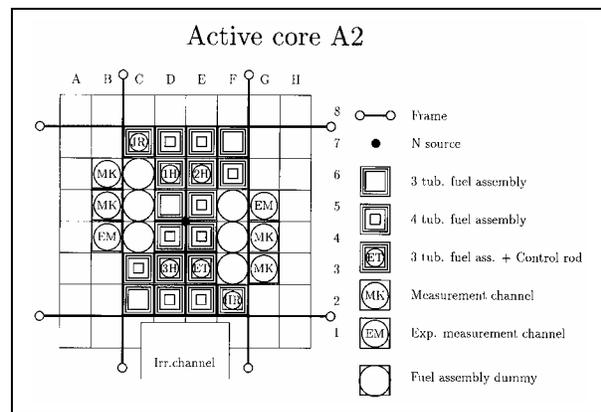
Fig. 7. Operational Core configuration A2
