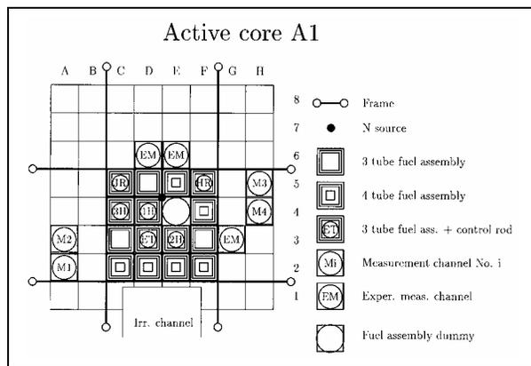
Fig. 6. Operational Core configuration A1
