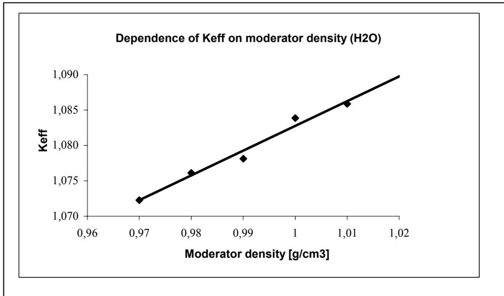
Fig. 4. Dependence of  $K_{eff}$  on moderator density (H<sub>2</sub>O)
