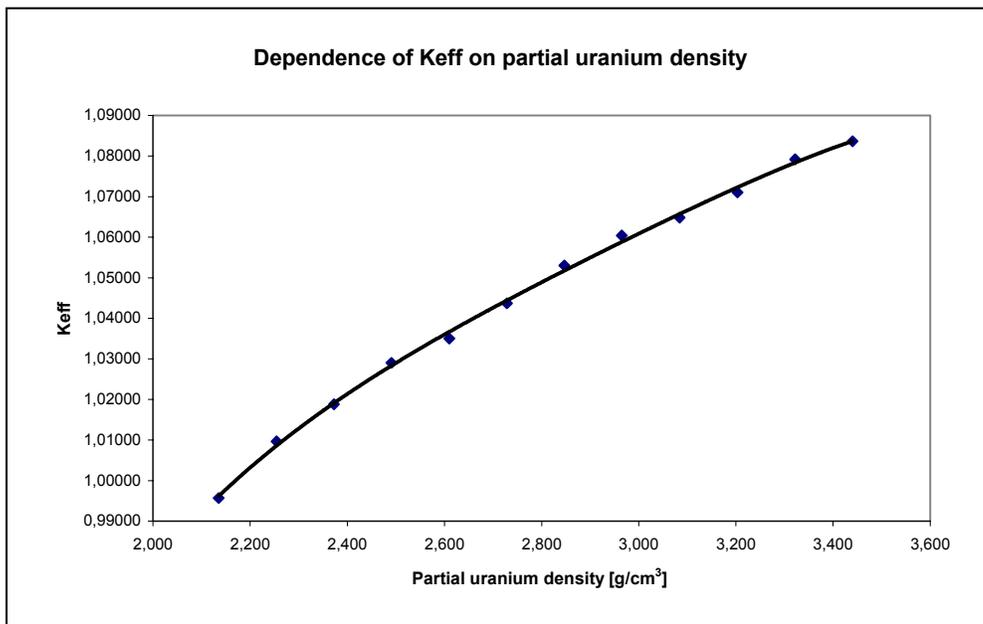
Fig. 3. Dependence of  $K_{\text{eff}}$  on partial uranium density
