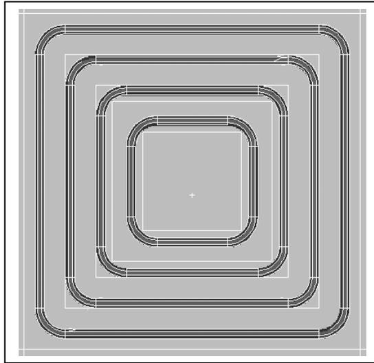
Fig. 1. IRT-2M Fuel assembly model in MCNP code
