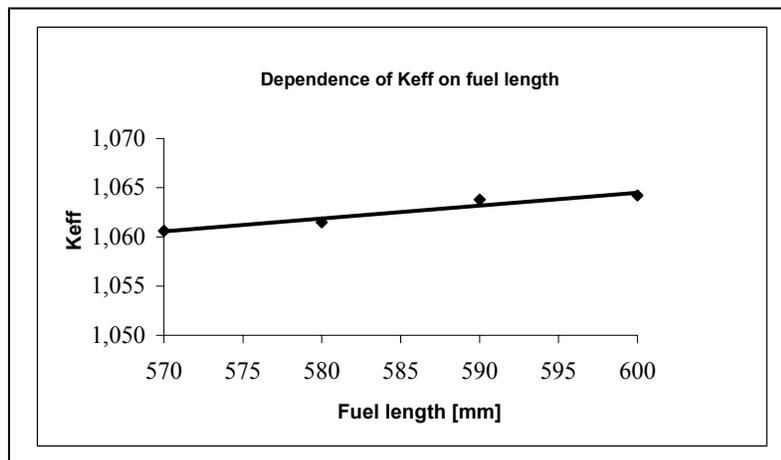
Fig. 5. Dependence of  $K_{eff}$  on fuel length
