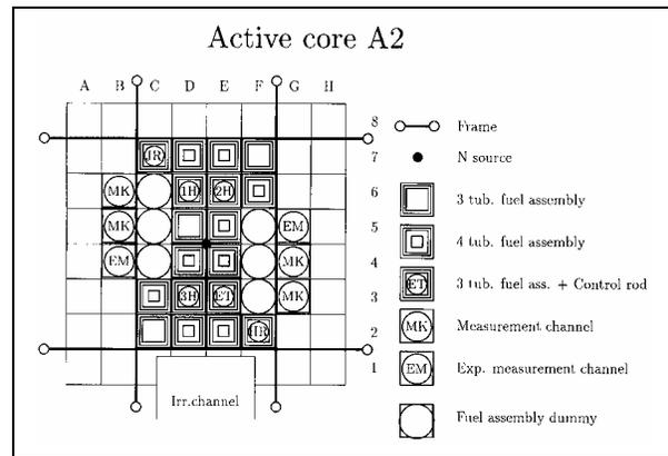
Fig. 7. Operational Core configuration A2
