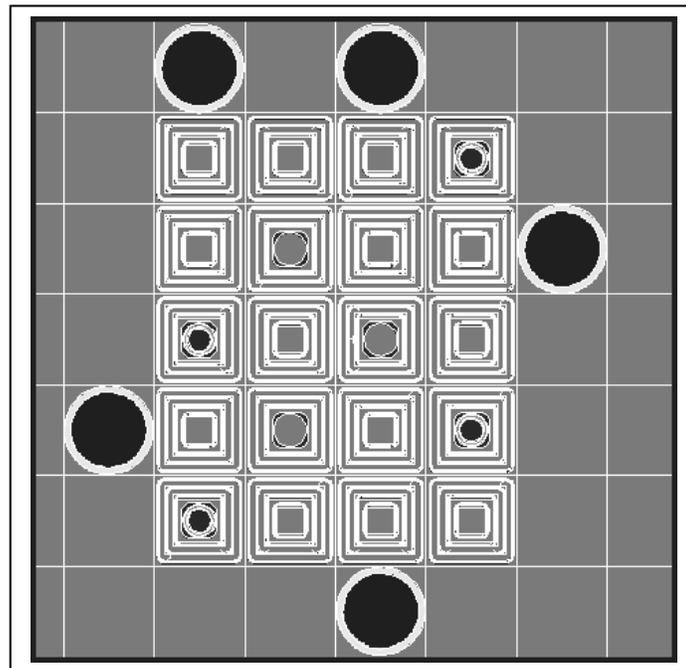
Fig. 2. Hypothetical Core configuration with 20 fuel assemblies
