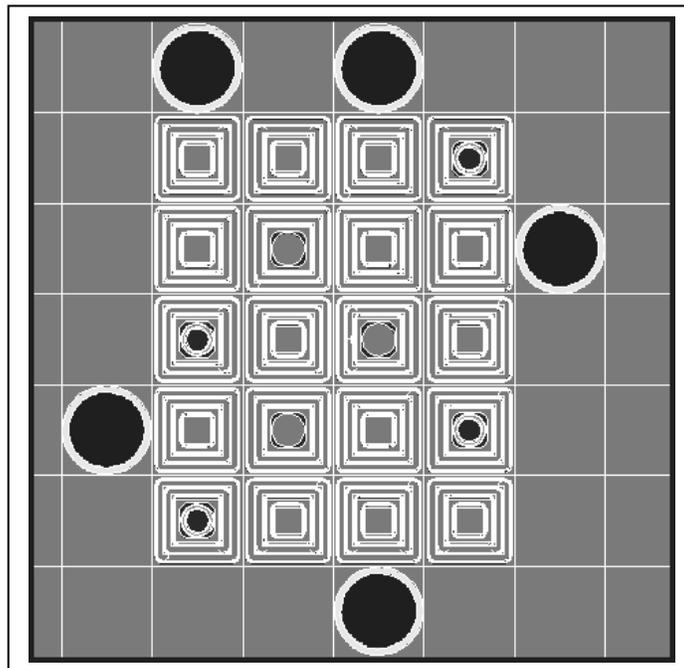
Fig. 2. Hypothetical Core configuration with 20 fuel assemblies
