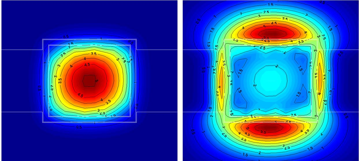
Fast flux ( $E > 0.907$  MeV, axial mean  $\times 10^{14}$  n/cm<sup>2</sup>/s)
