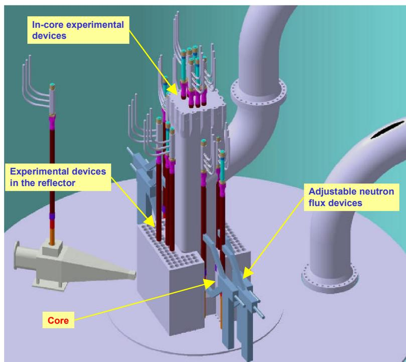
Reactor core and irradiation devices
