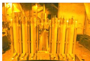
Fig.21: RRSF-canister 12-positions rack in dissolution cell
