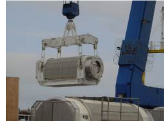
Fig.33: AREVA TN-28 transportation cask
