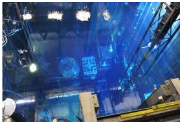
Fig.14: The baskets used for RRSF transfer to wet storage
