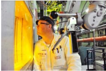
Fig.22: operator handling RRSF with tele-manipulator
