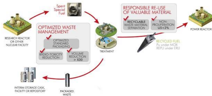
Fig. 1: RRSF reprocessing basic scheme and advantages
