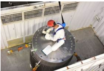
Fig.9: Radiological control on RRSF transportation cask, without shock absorber
