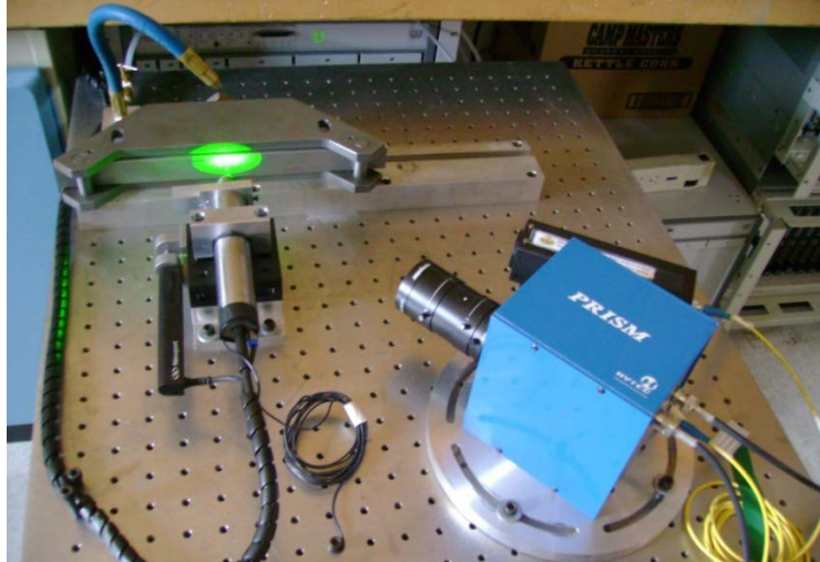
Figure 6. Setup for hole drilling tests showing calibration sample.
