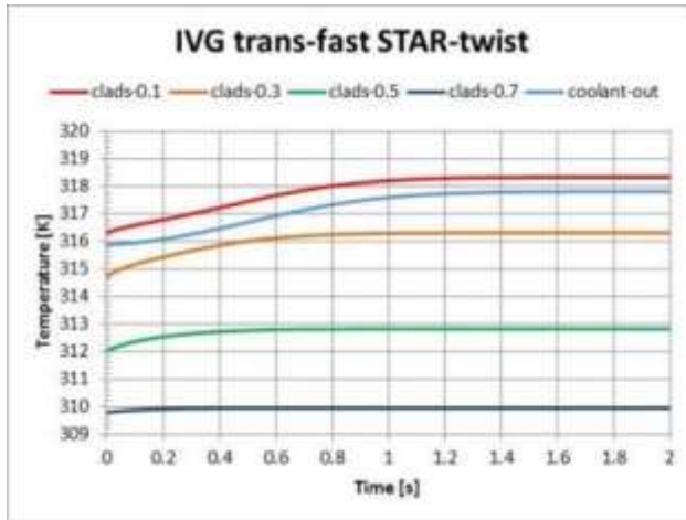
Fig. 4.3 Coolant Outlet and Clad Surface (0.1, 0.3, 0.5, and 0.7 m elevation) Temperatures Calculated Using STAR for Fast Transient
