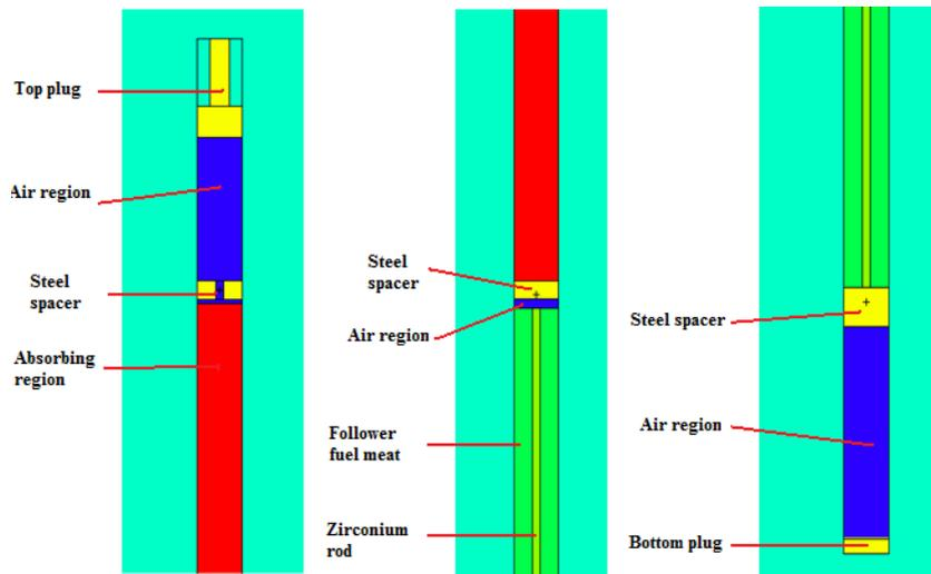
Figure 7. Model for the control rod with fuel follower.
