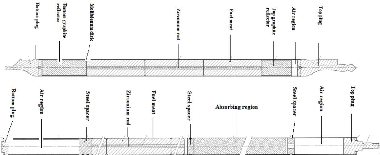
**Figure 5.** Fuel and the control rod schematic views.
