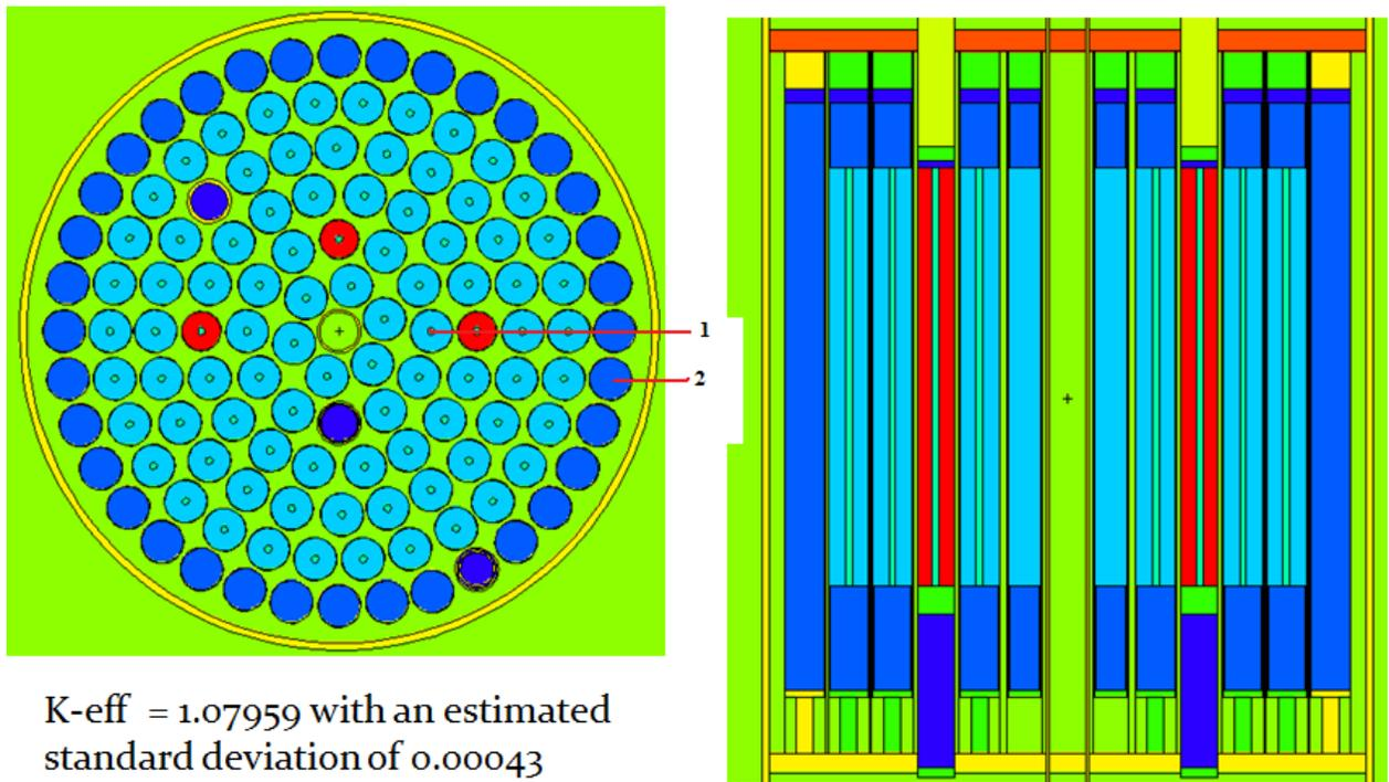
**Figure 8.** The reactor core with 85 fuels and three control rods fuel followers completely inside the core.
