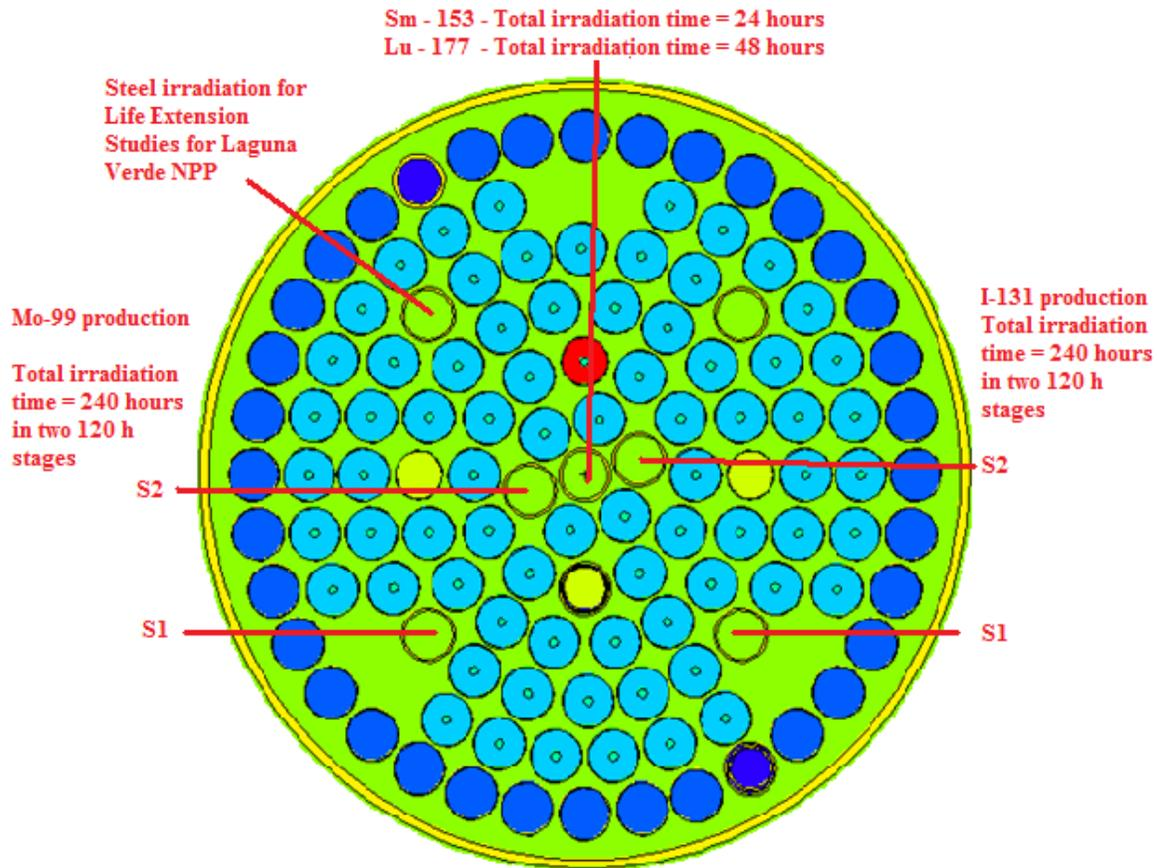
**Figure 10.** The selected design and the intended uses for the new in-core facilities.
