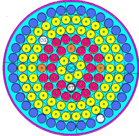
**Figure 4.** Reactor core with HEU and LEU fuel
