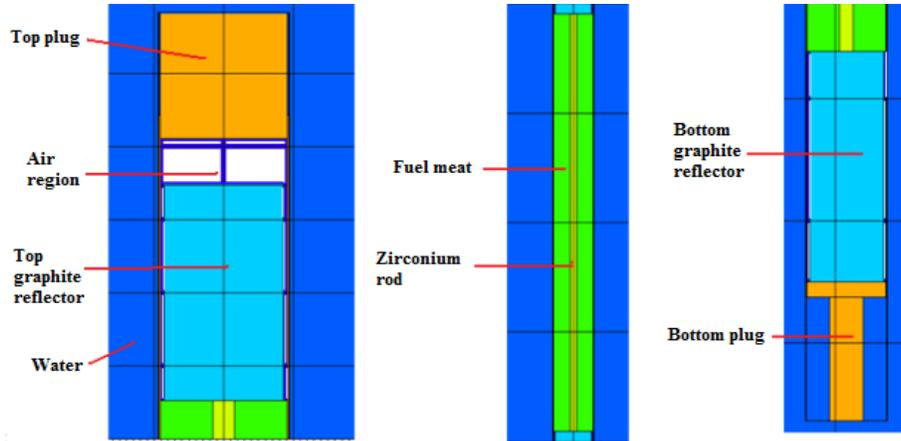
Figure 6. The model for the fuel.
