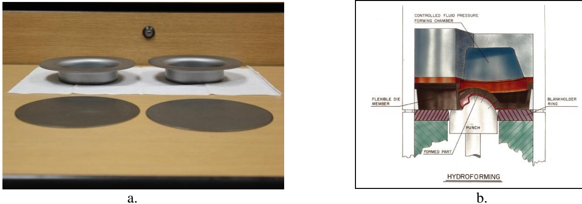
Figure 4 Example of a formed HIP can. a. Round formed HIP cans used to demonstrate feasibility b. Schematic of hydroforming press used to make round formed HIP cans. K. Clarke
