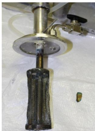
**Figure 12.** Anode basket and remaining U foil
