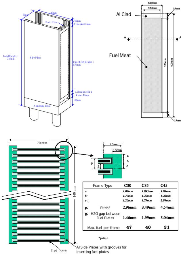
**Figure 6:** Structure of KUCA Light Water-Moderated Core (C-core) Flat Plate Fuel Elements
