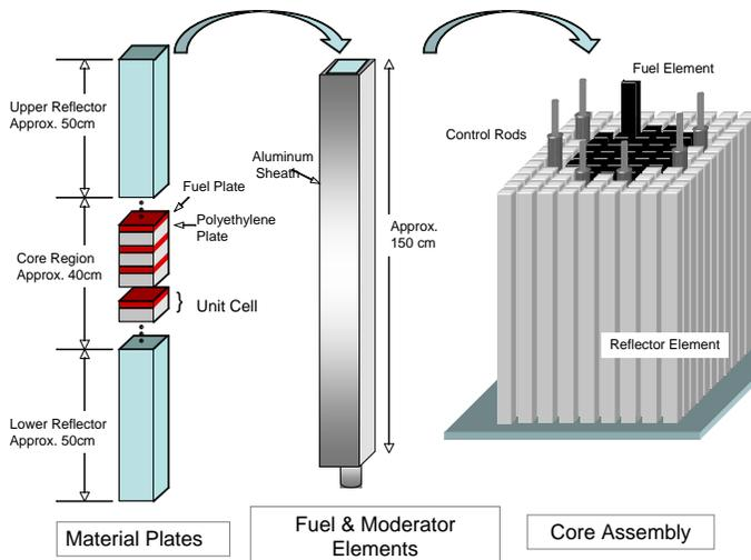
**Figure 3:** Schematic View of KUCA Solid-Moderated Core and Fuel Elements
