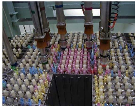
**Figure 4:** KUCA Solid-Moderated Core (B-core), showing fuel elements, control rods and removable section of the core (in shutdown position)
