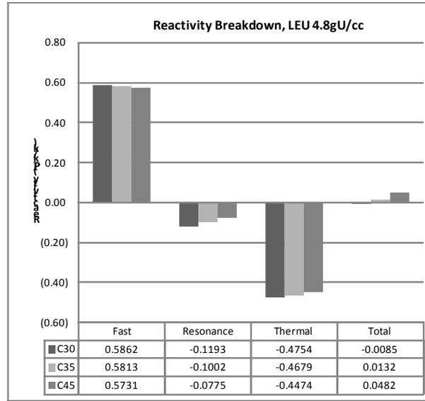
**Figure 10:** reactivity difference breakdown by energy region for LEU fuel, 4.8gU/cc
