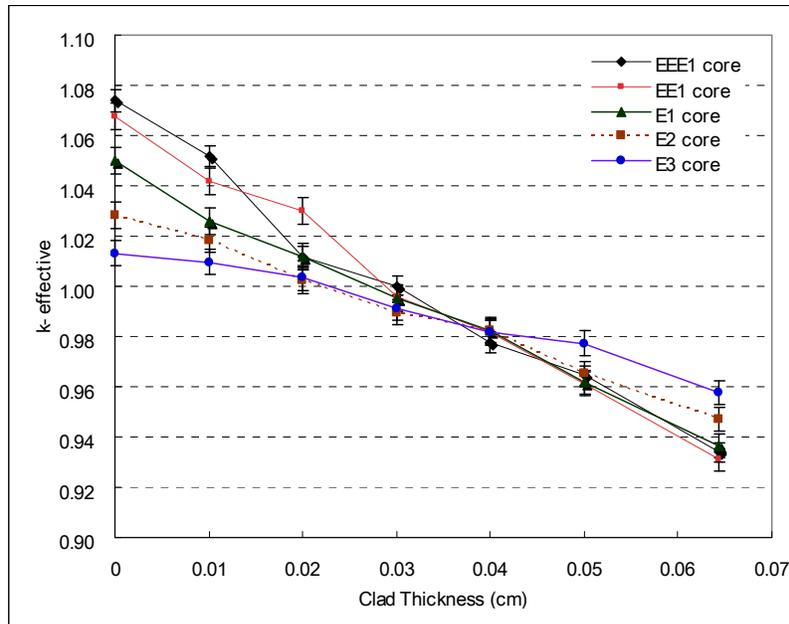
**Figure 14:** Criticality (k-effective) of dry cores with U-9Mo+Al clad
