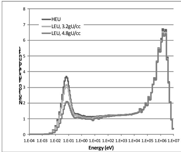
**Figure 7:** Comparison of C35 fuel cell neutron spectrum
