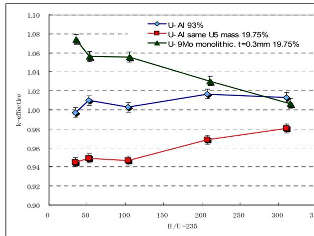
**Figure 13:** Comparison of k-effective for dry core using LEU
