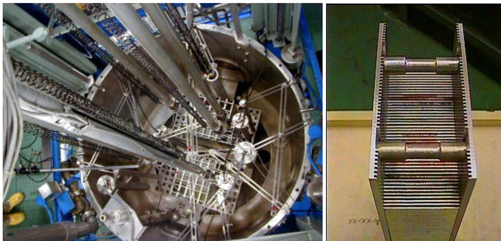
**Figure 5:** KUCA Light Water-Moderated Core (C-core), showing the core tank and fuel element
