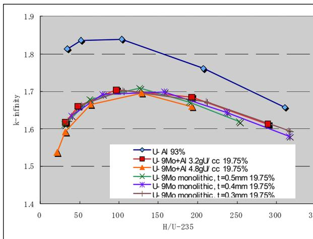
**Figure 12:** Comparison of k-infinity for dry core unit fuel cell using U-9Mo
