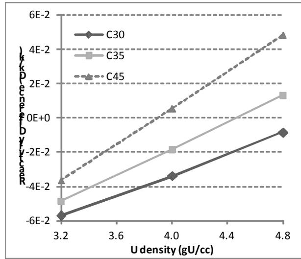
**Figure 8:** reactivity difference between HEU and LEU with various U density for C35 core
