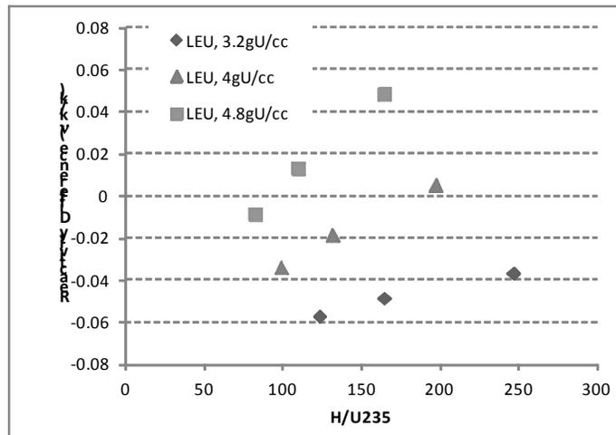
**Figure 11:** Change in H/U-235 ratio and Associated Reactivity Change due to LEU Utilization
