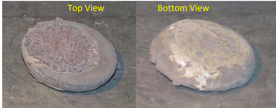
Figure 3. Uranium Consolidation Ingot
