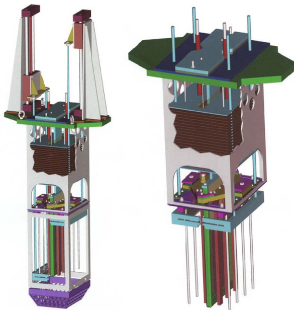
Figure 1. Sketch of ANL Planar Electrode Electrorefiner (PEER)
