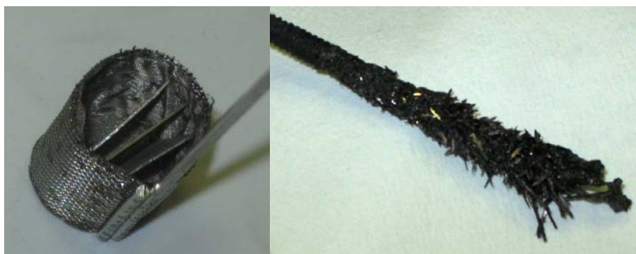
Figure 5. Loaded Anode Basket (Left) and Cathode Deposit (Right) from Irradiated Fuel Test
