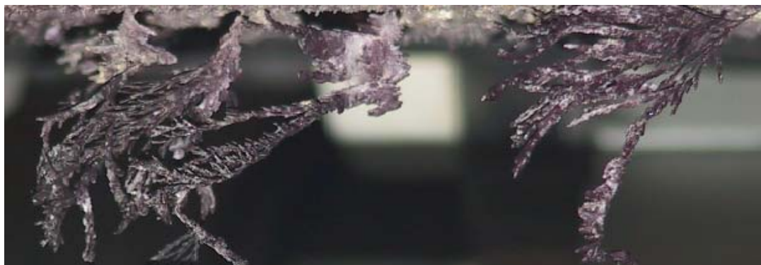
Figure 2. U-10Mo Scrap Uranium Deposit Adhering to Cathode Rods
