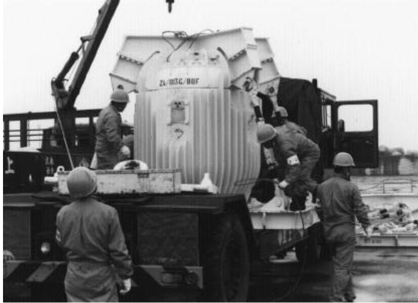
Figure 2. UNIFETCH-L Transporting Cask
