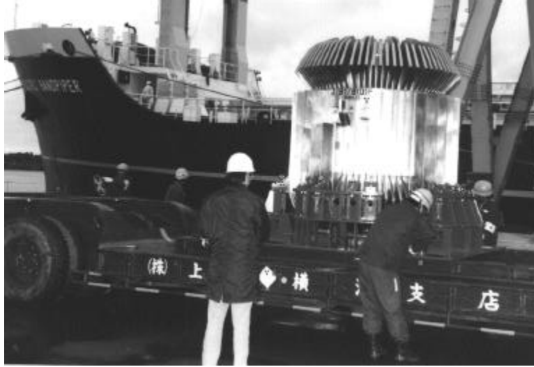
Figure 3. JRC-80Y-20T Transporting Cask
